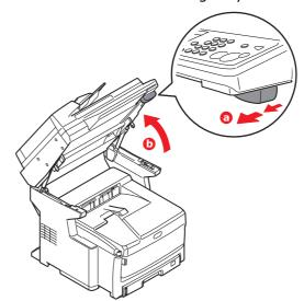
**3.** Press the cover release (a) and open the top cover (b) fully.
